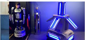
Unicorn was developed with some of the most advanced technologies — such as 5G, Artificial Intelligence, machine learning, IoT and cloud computing. For its disinfection capabilities, it comes equipped with ultraviolet-C (UVC)-emitting light, itself a widely used sterilisation technology, commonly found in hospital operating rooms to quickly inactivate a range of pathogens.
